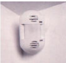
Occupancy and Light Level Sensors are often an excellent compliment to energy efficient lighting. With instant re-strike fixtures, light fixtures can be turned fully or partially off, only to be brought to full brightness when the room is occupied, or when daylight levels are not sufficient for the task. These strategies can add an additional 25 to 50 percent energy savings to a commercial lighting project.
