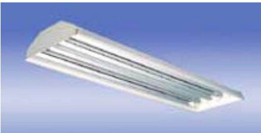
T-5 Electronic Ballast High Output Fixture – This fixture replaces high-bay HID fixtures in retail, manufacturing and warehouses. The 16" x 4' fixture with four T-5 lamps and a specular reflector uses only 234W to provide the light output of a 450W metal halide fixture (typical in Home Depot, Gymnasiums, Manufacturing). Other advantages over HID include instant re-strike, high color rendition (84 CRI vs. 60 CRI) and 95% lumen maintenance (only 5% light loss over
