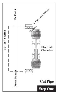
The *ECOsmarte Electrode Chamber* may be installed either between the pump and filter or, preferably, after the filter. The titanium electrodes should be aligned nearest the pool (see diagram). If you have a spa in line with your pool filter system, ensure the *Electrode Chamber* is located before the valves that divide return water to the pool and spa.
