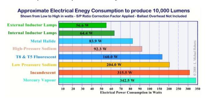
Looking at a real-world example, we can replace a 250W metal halide fixture with a 200W induction lamp based fixture, or even a 120W induction lamp fixture, thereby reaping a considerable saving in energy costs.
