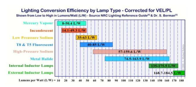
Induction lamps have the highest energy conversion efficiency once the correction factor is applied (as they have a high S/P ratio of 1.96 or 2.25 depending on model). Induction lamps are therefore a better choice as they produce more light useful to the human eye (VEL/PL) while using less electrical energy.
