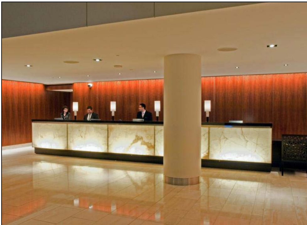
Figure 2.25. Registration Desk area with LED accent and wall-grazing (onyx panels are backlighted with fluorescent lamps, and the pedestal lights use incandescent lamps). www.kenricephoto.com
