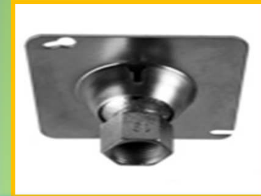
Swivel pendant mount square plate with a ball that allows fixture to hang straight (mount to standard electrical box; \frac{3}{4} " conduit) SPMSP
