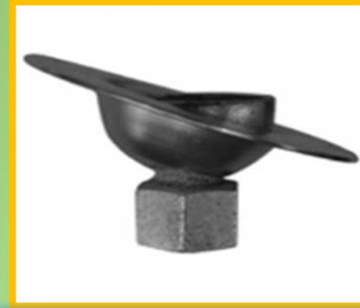
Swivel pendant mount round plate with a ball that allows fixture to hang straight (mount to standard electrical box; \frac{3}{4} " conduit) SPMRP
