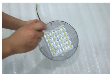
①Unscrewing four pieces screws in the lamphead.
