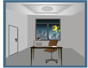
After stand-by period, the sensor switches off the lamp if no motion is detected in its detection zone.
