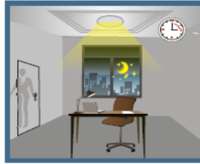
After hold time, the sensor dims the lamp at a low light level if no new motion trigger.
