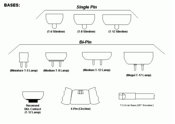
Mini Bi-Pin base is used mostly for T5 diameter tubes. It is a smaller version of the MBP contact base.
