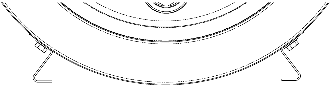
Solar Storage Tank with Z-section Feet (Rheem Hiline 52S tanks and Sunheat direct 'D' tanks)
