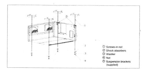
Once all these operations have been completed, the false ceiling to hide the unit may be installed, but a register cover must be left below for future maintenance. Grills of an adequate size should be incorporated in the unit for return air suction.
