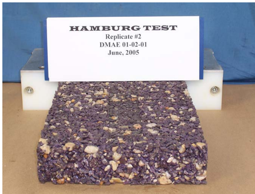
Hamburg Loaded Wheel Tester, 8,000 cycles @ 60°C – Replicate 2
