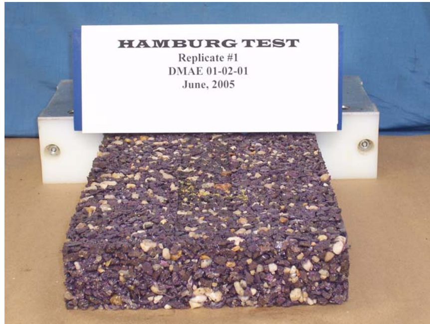
Hamburg Loaded Wheel Tester, 8,000 cycles @ 60°C – Replicate 1
