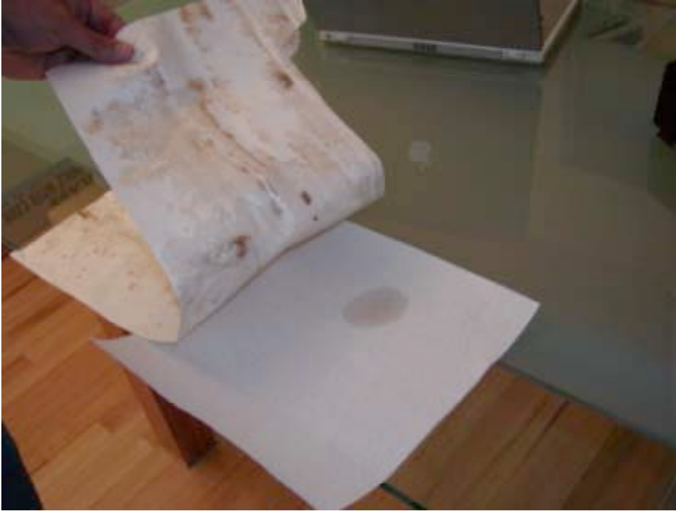
Photograph 7: Absorptive Surface For Water Drop Test
