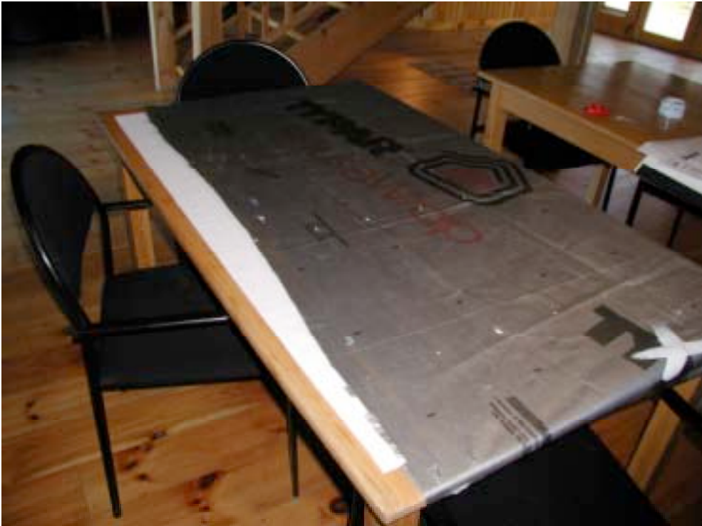
Photograph 9: Extensive Failure of Plastic Housewrap During Water Drop Test
