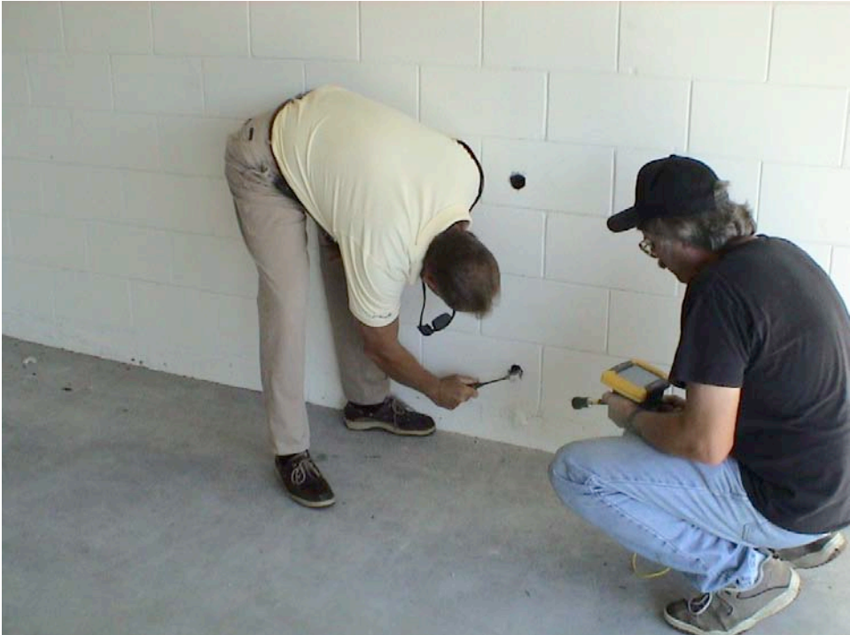
Photograph 47: Access Openings In Mass Wall – Camera Probe Leak Detection
