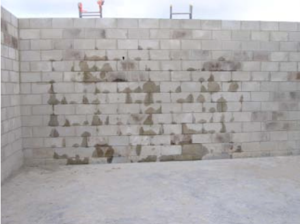
Photograph 57: Spray Rack – Unpainted Stucco Rendering
