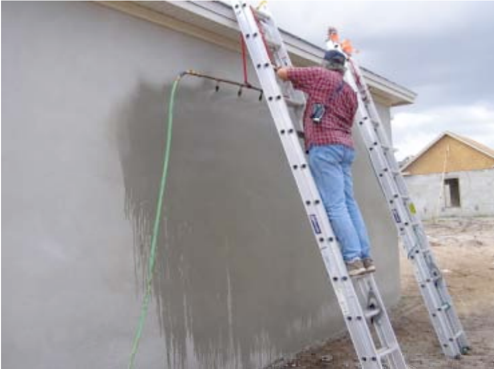
Photograph 57: Spray Rack – Unpainted Stucco Rendering
