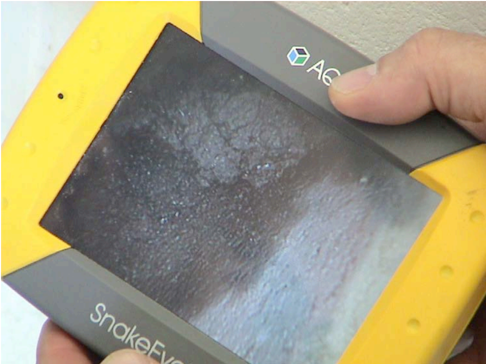
Photograph 47: Access Openings In Mass Wall – Camera Probe Leak Detection
