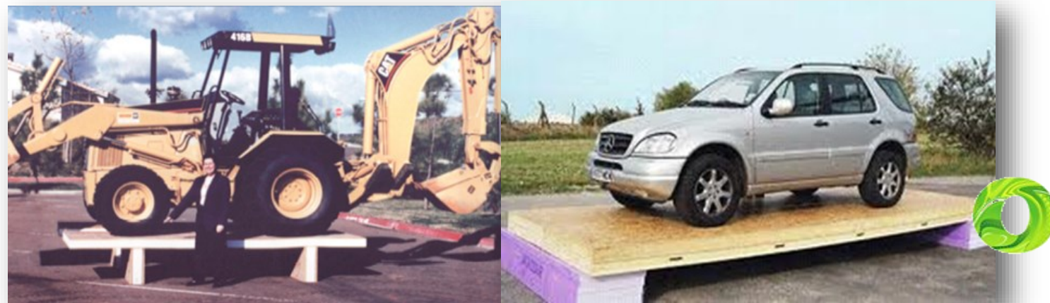
SIPs support bending loads like a beam
