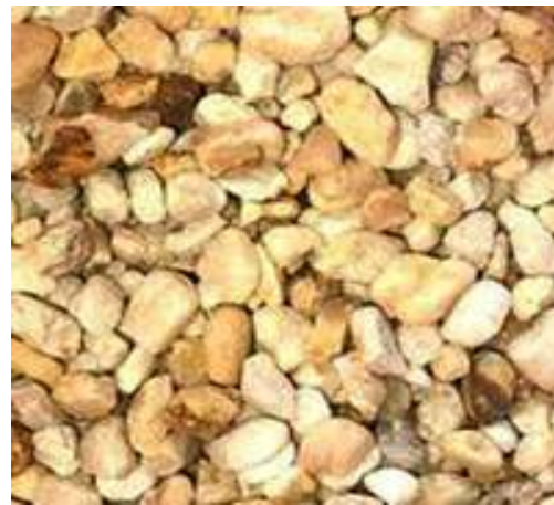
TRIPLE WASHED AND KILN DRIED STONE AGGREGATE.
